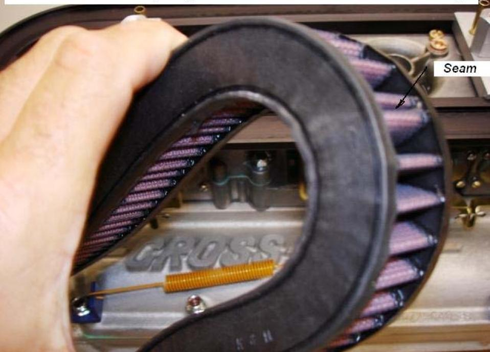
Place the filter in the base ensuring that the filter element is in the retaining gland
