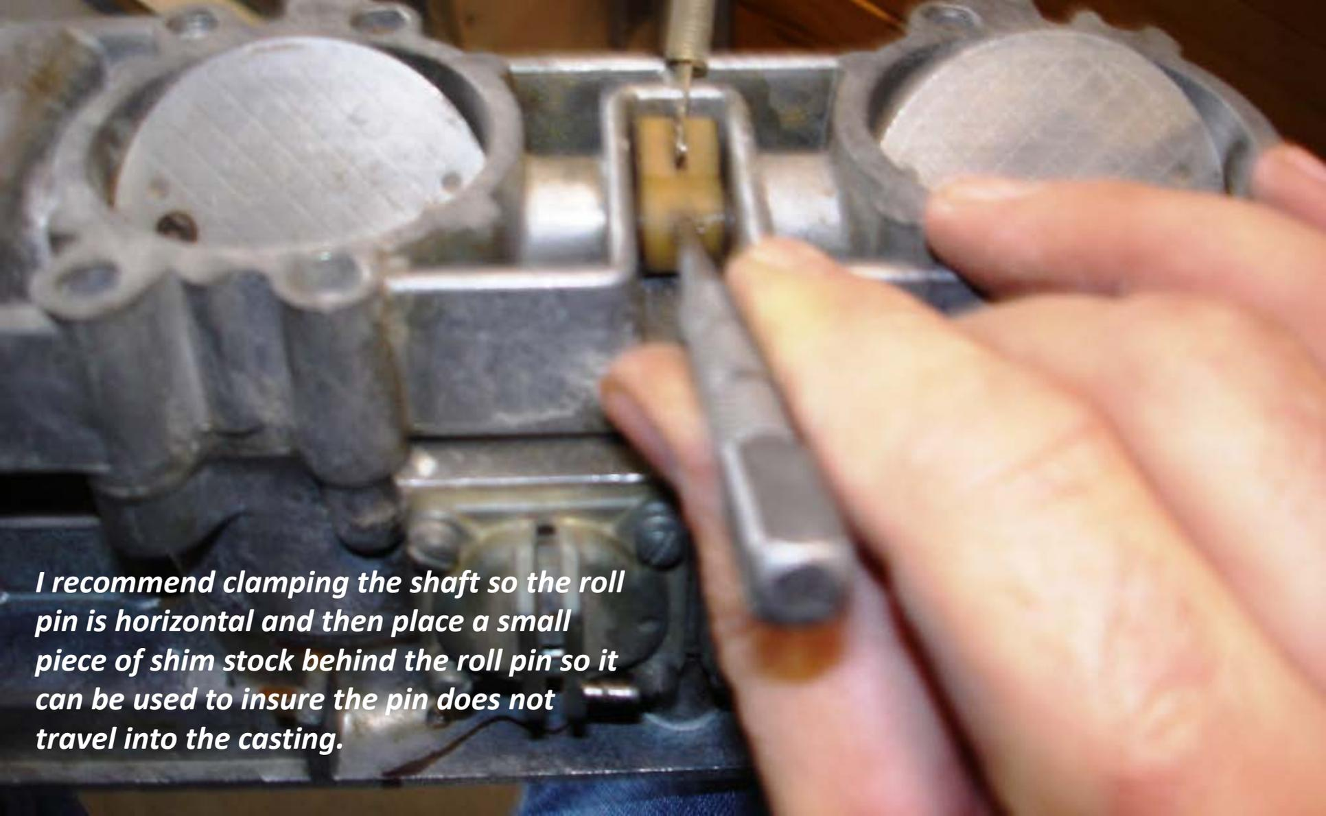
*If the pin is driven too far, you will be very unhappy. I had this happen to me once many years ago and have about five carbs sent to me with the pin driven down into the corner of the casting as shown. There is no saving th Nylon drive arm at this point as it must be broken to get at the roll pin, which is of course too hard to be nipped with cutters but the space is too confined to get in their with anything substantial enough to make the roll pin surrender.*
