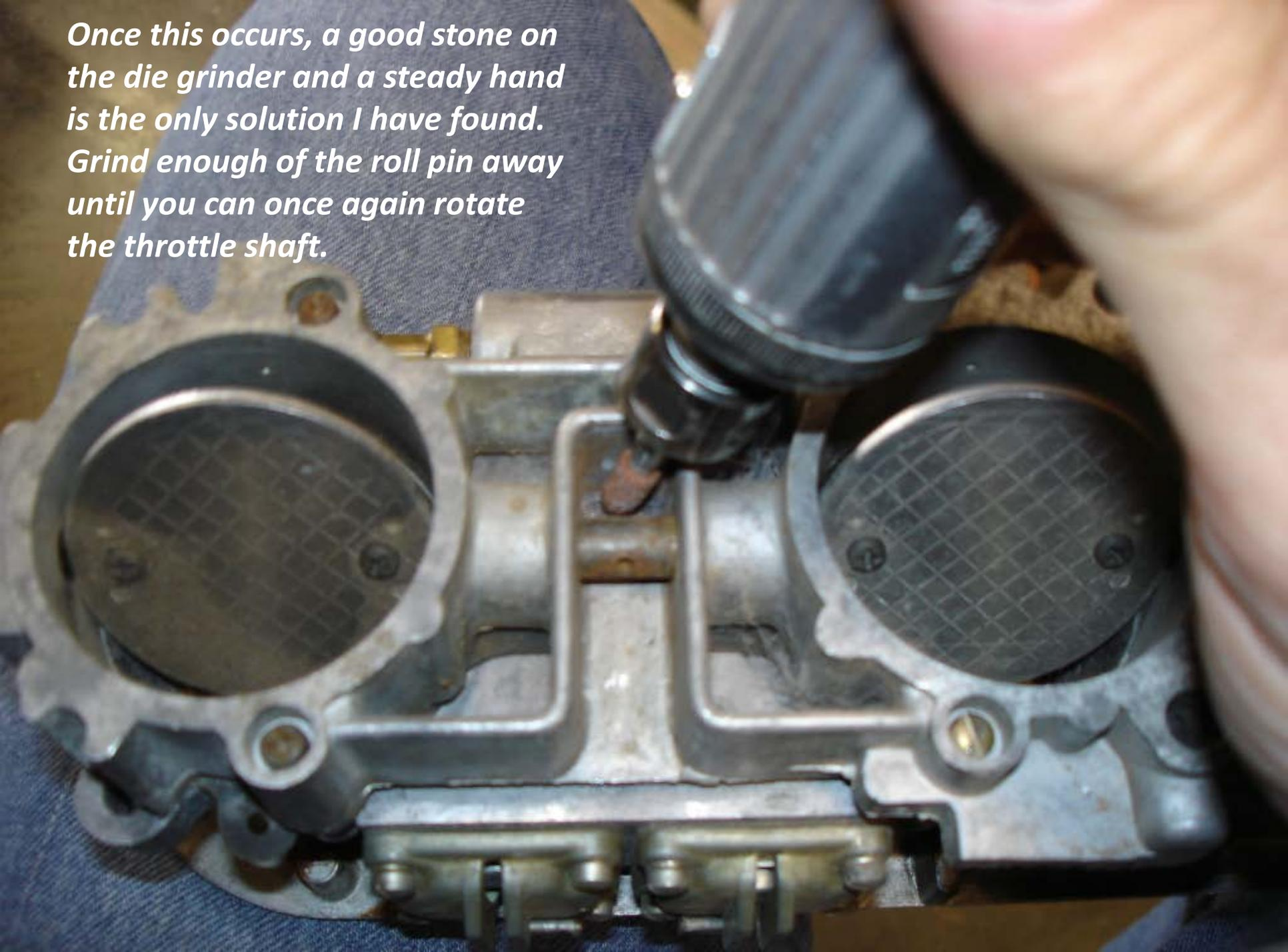
*After grinding away enough of the roll pin, you can either punch it through or rotate the shaft and grab it with a pair of needle nose vise grips and pull it out of their.*
