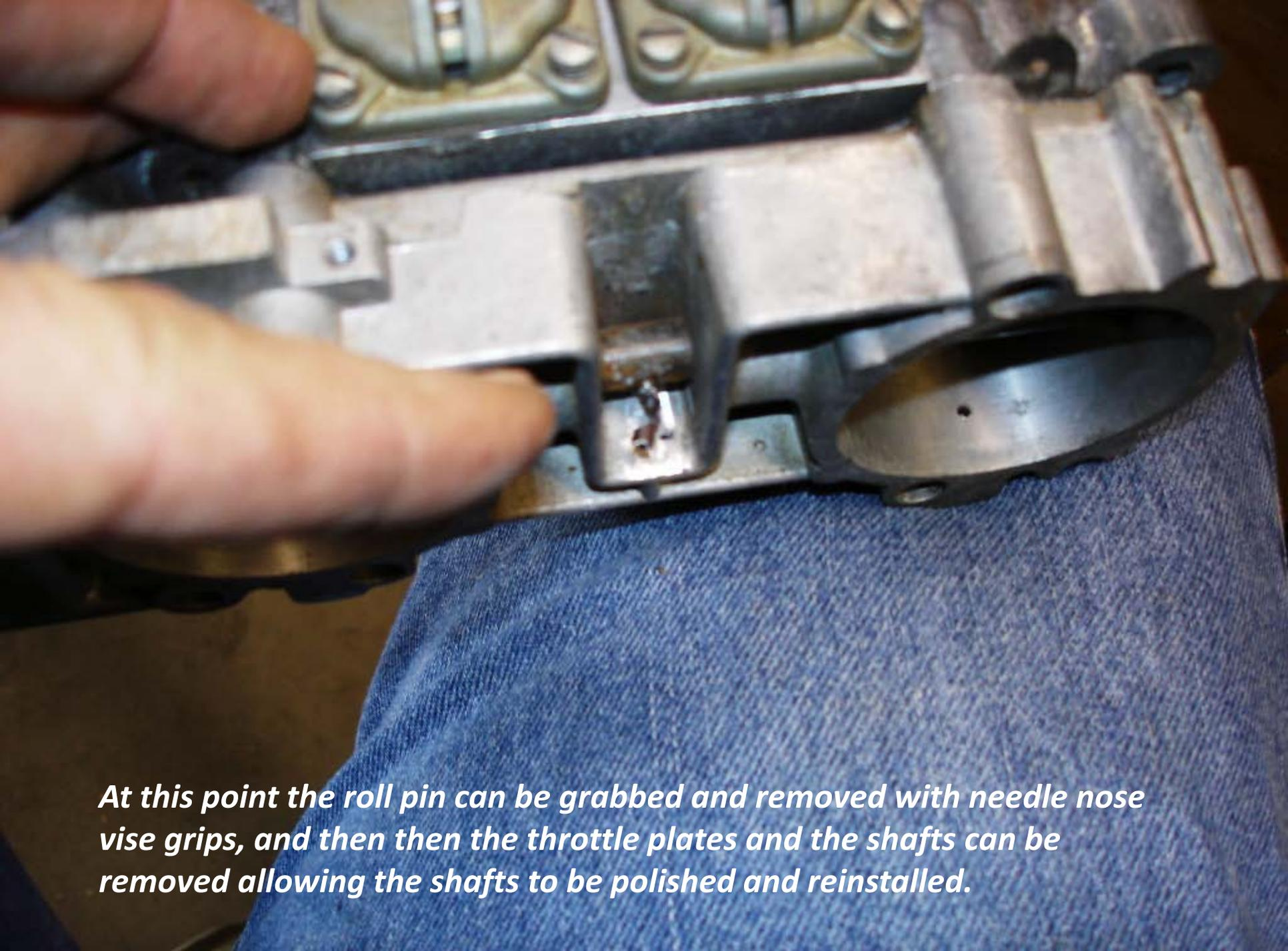
*At this point the roll pin can be grabbed and removed with needle nose vise grips, and then then the throttle plates and the shafts can be removed allowing the shafts to be polished and reinstalled.*
