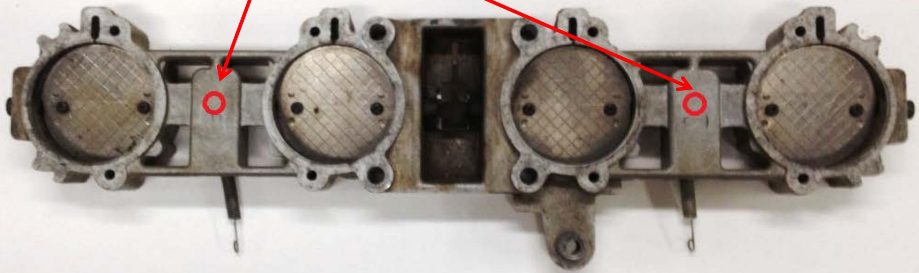
*This is the direction you must drive the roll pin but be very careful not to drive it too far. If you do, you will not be able to rotate the shaft due to the roll pin interfering with the casting. This is how you become a customer for my billet drive levers because the only way to get to the roll pin is to break off the nylon drive lever and grind away the hardened pin.*
