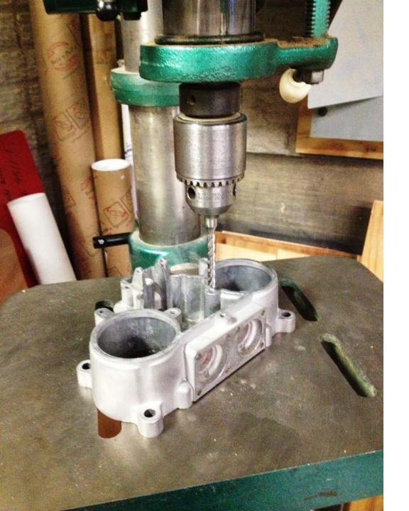
I recommend using an end mill to make the mod described on the previous slide because it cuts crisp flat bottom hole and a good edge to coin the check valve seat. Set of 4 conical accelerator pump check valves included with installation instructions.
