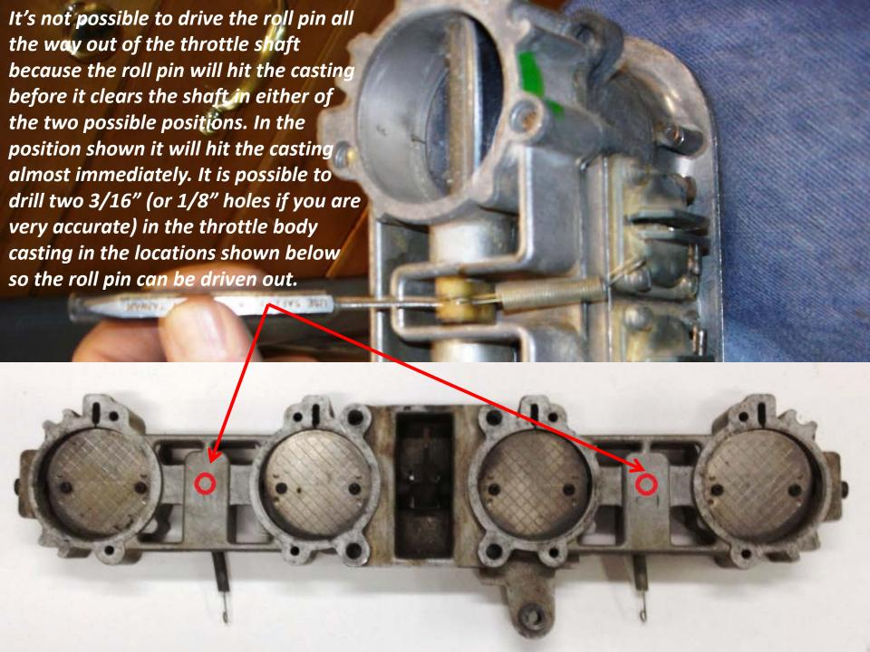
This is the direction you must drive the roll pin but be very careful not to drive it too far. If you do, you will not be able to rotate the shaft due to the roll pin interfering with the casting. This is how you become a customer for my billet drive levers because the only way to get to the roll pin is to break off the nylon drive lever and grind away the hardened pin.
