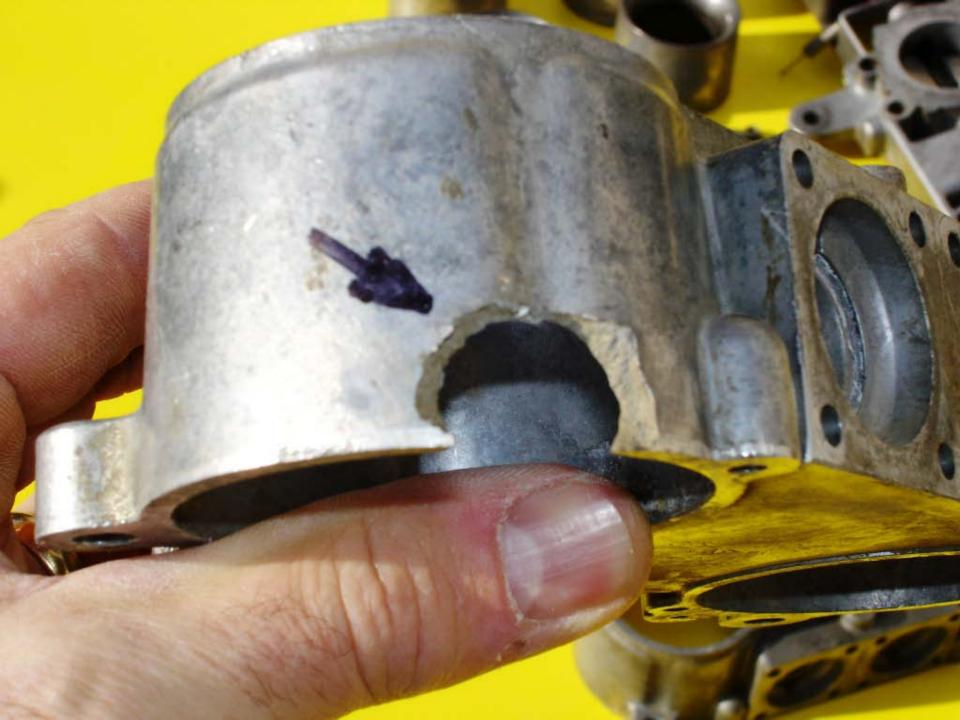
Relieve inside edge of crack for better weld penetration
