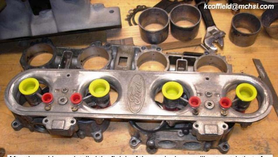
After the welds are detailed the finish of the worked area will not match that of the oxidized casting. To improve cosmetic appearance and gain a consistent finish the entire casting surface needs to be worked. Media blasting is an option but will leave a rough finish that easily stains. Polishing is an option but tedious. I prefer vibratory media because it provides a uniform color a smooth finish that cleans up easily. It does take considerable effort to do properly.
