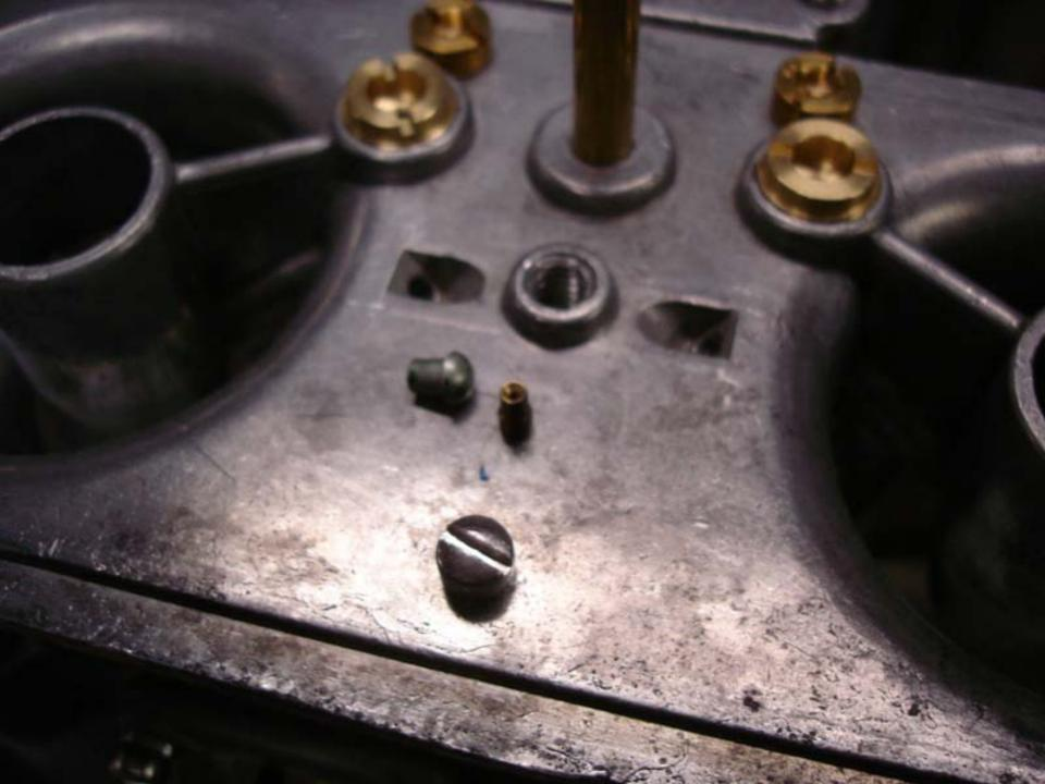
Now install new shooter and gently tap with a good fitting punch until the shooter is just at the edge of the air horn casting. Install a new rivet to seal the deal and you're done. If you do not have a rivet, alternately I have seen the opening drilled and tapped for a set screw., used along with some thread sealant
